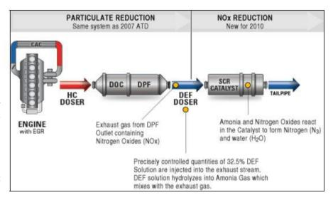
injects a fine mist of diesel into the exhaust stream. This mist then enters the DOC and reacts with a catalyst material. The result is a high heat output that is used to clean the DPF filter through a process called active regeneration. The HC doser does not operate continuously. It only operates when sensors indicate that the DPF filter needs to be cleaned and the vehicle is allowed to go into active regeneration mode.
