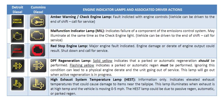
These indicators and warnings will display in a sequential order, indicating the degree of soot accumulation in the DPF and the urgency of performing regeneration. The diagram below shows the sequence of warnings and the available resolutions.
