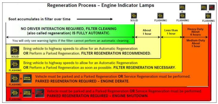
Note that when the DPF Regeneration Lamp is illuminated by itself (solid or flashing), the driver has the option of performing an automatic regen through uninterrupted highway driving or initiating a parked regen.
