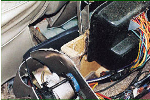
Note how the reciprocating saw cut through all materials encountered on the van in Plano.
